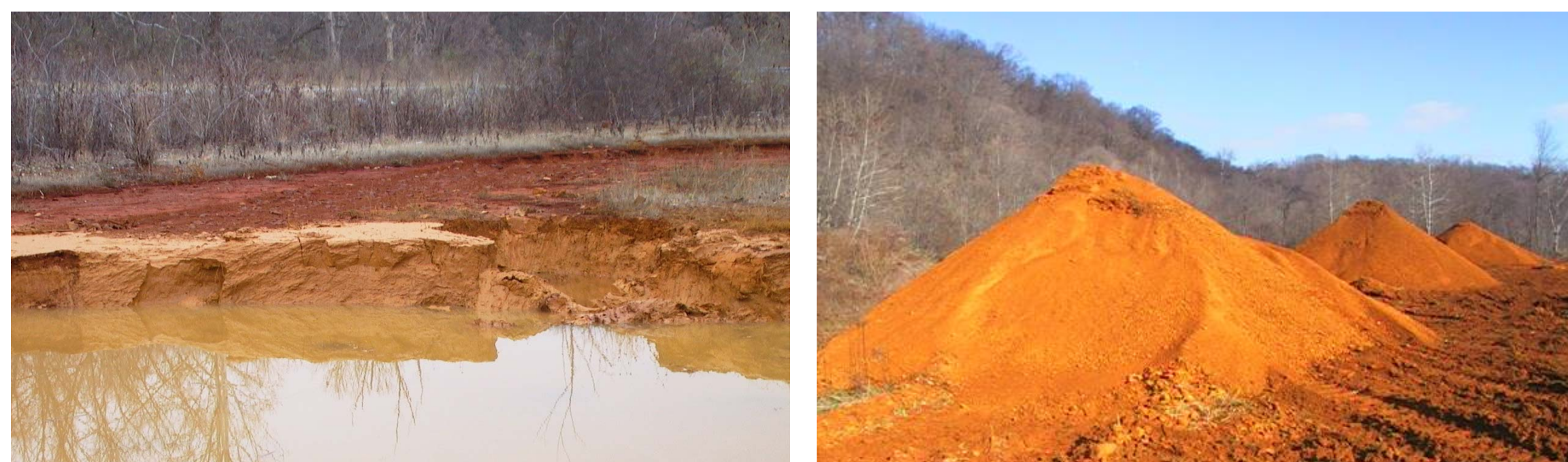
MDRs from a mine drainage treatment system during recovery (left) and after processing (right).
